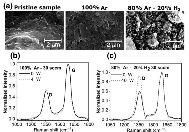
FIG. 5. (a) SEM micrograph of graphene surfaces. Left: Pristine sample. Center: After 5 min of 100% Ar plasma exposure. Right: After 5 min of 80% Ar – 20% H<sub>2</sub> plasma exposure. (b) Raman D and G peaks during no plasma and 100% Ar plasma exposure. (c) Raman D and G peaks during no plasma and 80% Ar – 20% H<sub>2</sub> plasma exposure.
