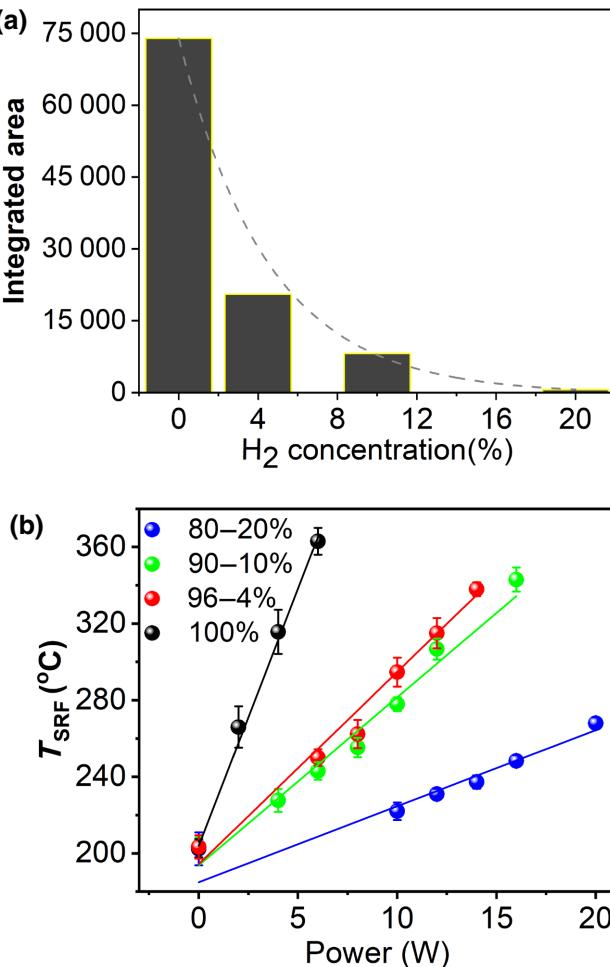
FIG. 4. (a) Integrated area of OES peaks as a function of H<sub>2</sub> dilution concentration in Ar. (b) Temperature at the graphene surface as a function of plasma coupled power for different Ar-H<sub>2</sub> gas concentrations.
