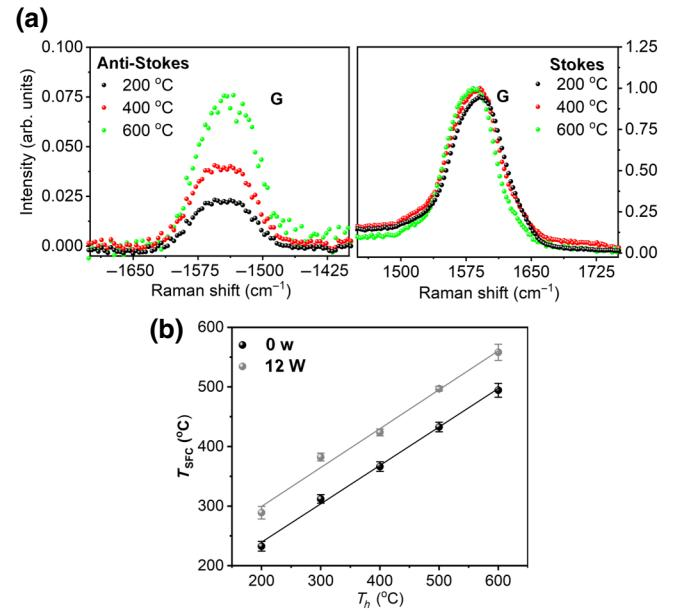
FIG. 2. (a) Anti-Stokes and Stokes *in situ* Raman G peak of multilayered graphene heated up at substrate temperature or 200 °C, 400 °C, and 600 °C, with plasma off, with a total flow of 30 sccm of an argon-hydrogen mixture. (b) Temperature at the graphene surface as a function of chamber temperature with and without a 12-W Ar-H<sub>2</sub> plasma, obtained by Raman thermometry.
