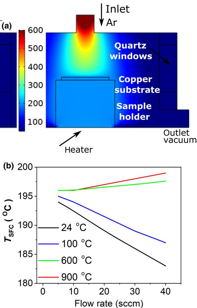
FIG. 3. (a) Heat transfer computer model in COMSOL MULTIPHYSICS to study the temperature profile at the substrate surface due to gas heating. (b) Calculated surface temperatures as a function of the flow rate for different gas temperatures.
